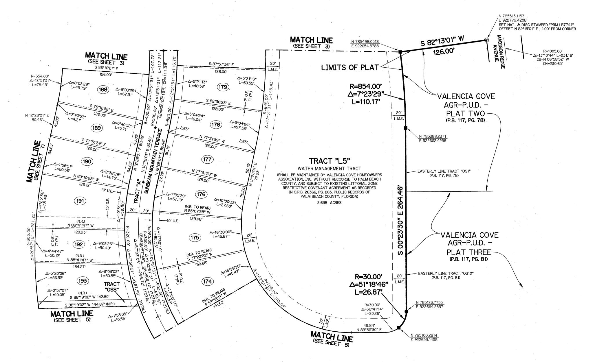
COORDINATES SHOWN ARE GRID COORDINATES DATUM = NAD 83 (1990 ADJUSTMENT) ZONE = FLORIDA EAST ZONE LINEAR UNIT = U.S. SURVEY FEET COORDINATE SYSTEM = 1983 STATE PLANE TRANSVERSE MERCATOR PROJECTION ALL DISTANCES ARE GROUND SCALE FACTOR = 1.0000240 PLAT BEARING = GRID BEARING
